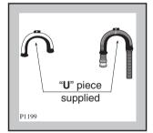
TPlace the drain hose into your standpipe, which should have an internal diameter of approximately 38mm thus ensuring there is an air break between the drain hose and standpipe.
